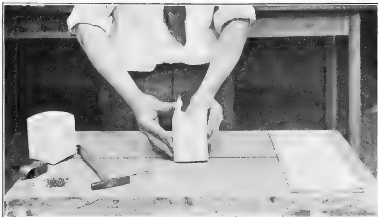
FIG. 10. — The paper is being folded over the top of the block in preparation for the use of a tack.
